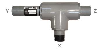
The aspirator conveys material pulled into the inlet (Y) side and conveys the material away from the area via the exhaust (Z) employing an attached conveyance hose. The system is powered by a ring compressor that introduces air pressure to the aspirator motive (X).
