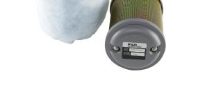
Fuji Electric Inlet Filters are designed to protect Ring Compressors by filtering the inlet air when used for pressure applications. The filter has a perforated outer cylinder and an inner liner wrapped with a fine mesh (.009) screen. The filter itself is rated for 200-micron filtration.
