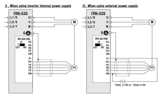
Figure 9 Connection Diagrams for Speed Control
