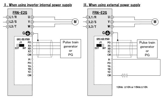
Figure 8 Connection Diagrams for Pulse Train Input
