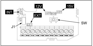
Note To move a switch slider, use a tool with a narrow tip (e.g., tweezers). Be careful not to touch other electronic parts, etc. If the slider is in an ambiguous position, the circuit is unclear whether it is turned ON or OFF and the digital input remains in an undefined state. Be sure to place the slider so that it contacts either side of the switch.
