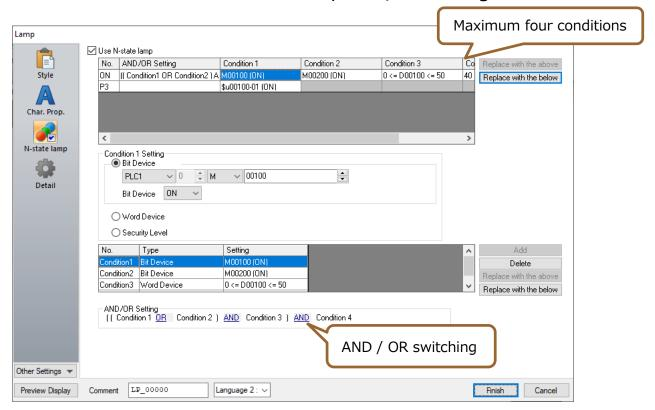
N-state lamp function is available for not only lamp parts but also switch parts.
