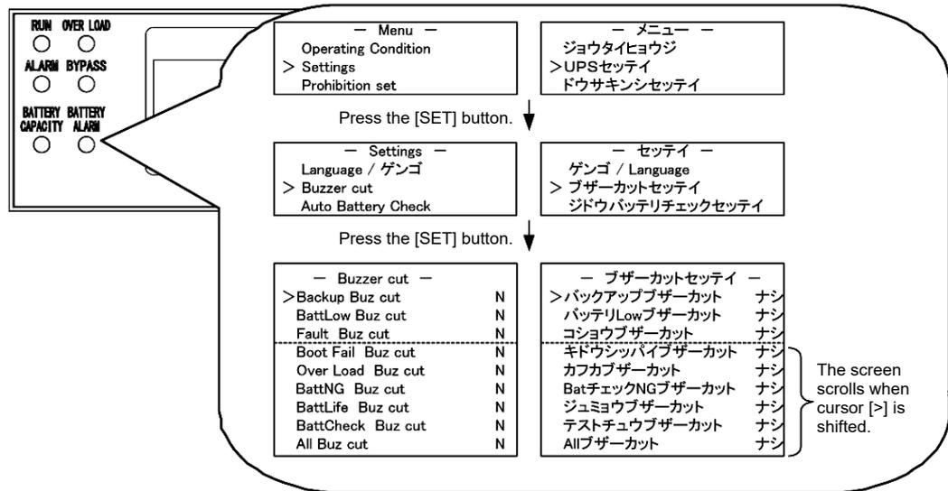
(5) Use the direction buttons (▼ button or▲ button) to select the target items.
