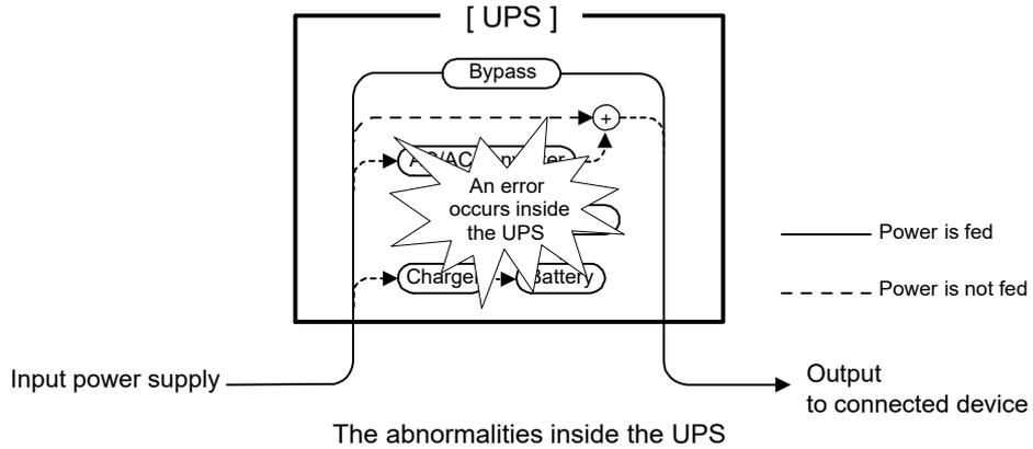
Electricity flow during automatic bypass operation
