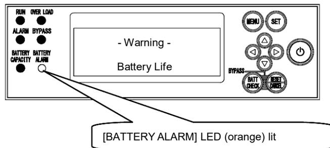
When the backup time of the battery has been lowered to 3 minutes or less (at the rated load)
