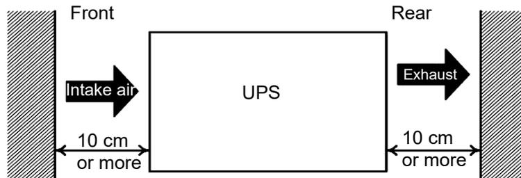
When performing maintenance on the UPS, a space of approximately 1 m is required in front of and behind the UPS.
