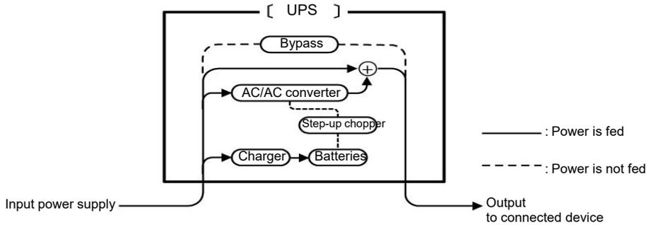
Electricity flow during normal operation
