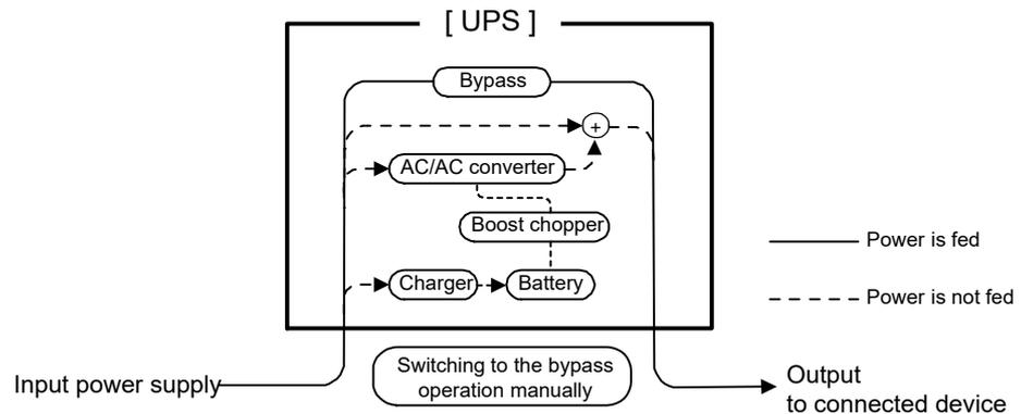
Electricity flow during automatic bypass operation
