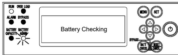
5. If no error was found in batteries during battery check for 5 seconds, and [BATTERY CAPACITY] LED on the front face of the Product shows the extent of battery charge (green) again, and return to the normal running status arises.
