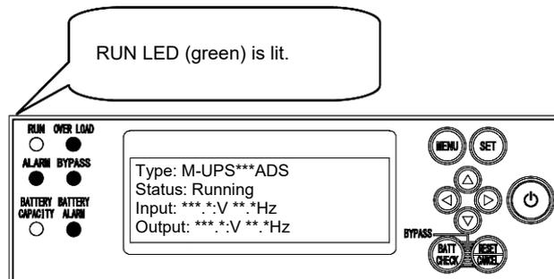
When all the LEDs on the front of the UPS are off, turn on the UPS and proceed to step 2. For details, refer to Chapter 4.1 "Turning on the UPS". Also refer to Chapter 7 "Troubleshooting".
