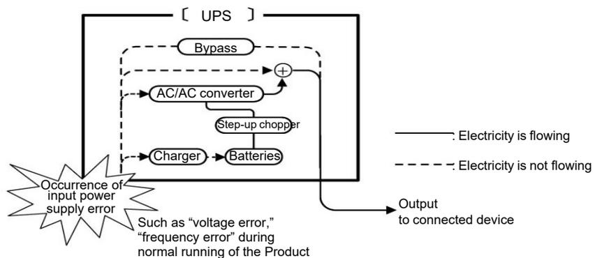
Electricity flow during battery operation
