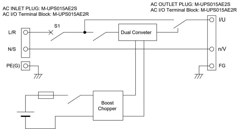
Fig 2. M-UPS030AE2 circuit diagram
