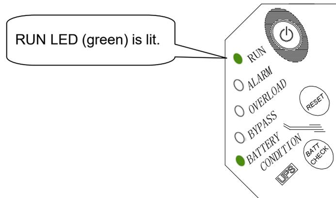
When all the LEDs on the front of the UPS are off, turn on the UPS and proceed to step 2. For details, refer to Chapter 4.1 "Turning on the UPS". Also refer to Chapter 6 "Troubleshooting".
