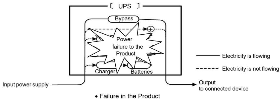
Electricity flow during automatic bypass operation
