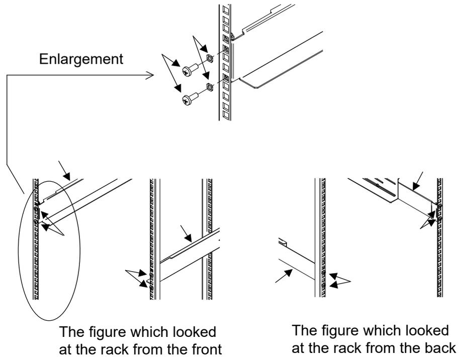
3. Put the system on the rail, and fix the right and left in the front side part with screws for rack mounting .
