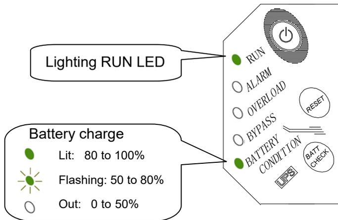
4. The battery check is performed automatically.
