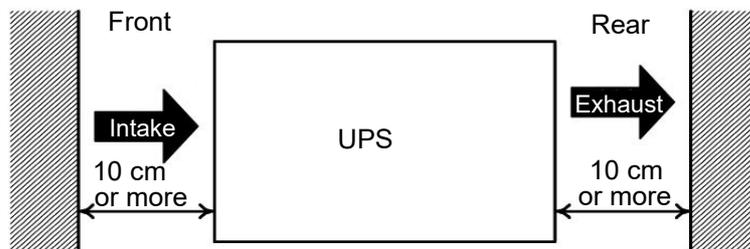
When performing maintenance on the UPS, a space of approximately 1 m is required in front of and behind the UPS.
