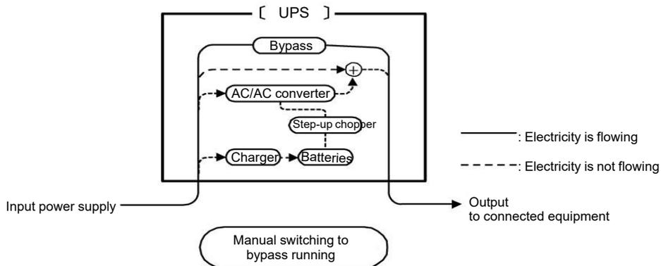
Electricity flow during manual bypass operation
