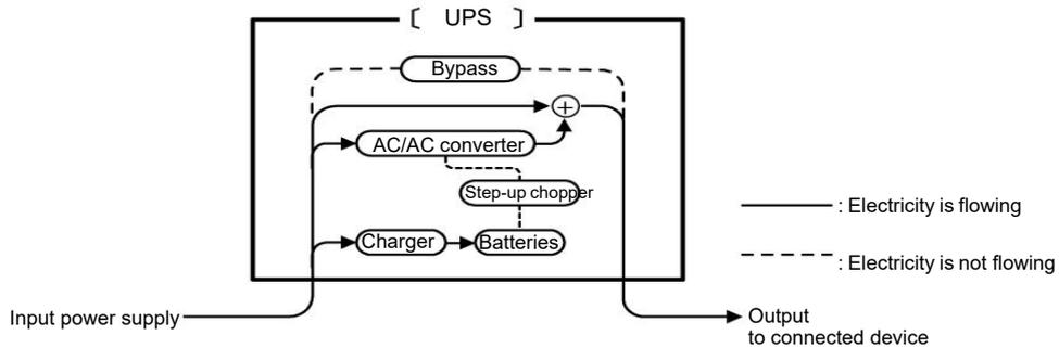
Electricity flow during normal operation
