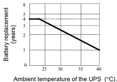
Relation between the ambient temperature and the cycle of battery replacement
