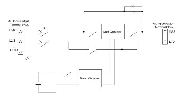
Figure 2 - Circuit diagram of Models M-UPS075AD2B-U and M-UPS100AD2B-U
