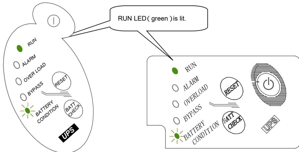
When all the LEDs on the front of the UPS are off, turn on the UPS and proceed to step 2.
