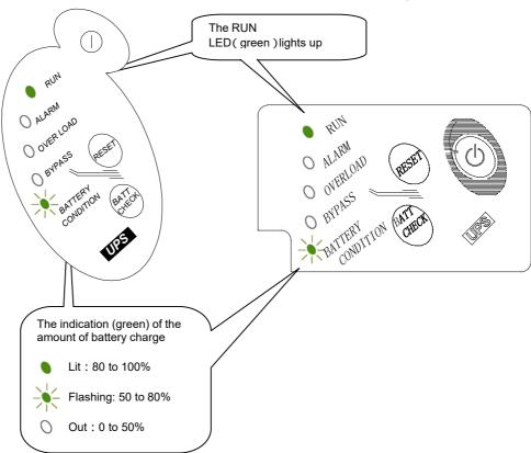
**4.** The battery check is performed automatically. The BATTERY CONDITION LED (orange) on the front of the UPS flashes (in the cycles of 1.6 seconds).
