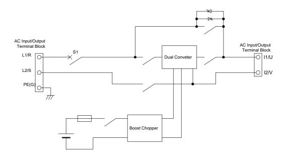
Figure 1 - Circuit diagram of Model M-UPS050AD2B-U
