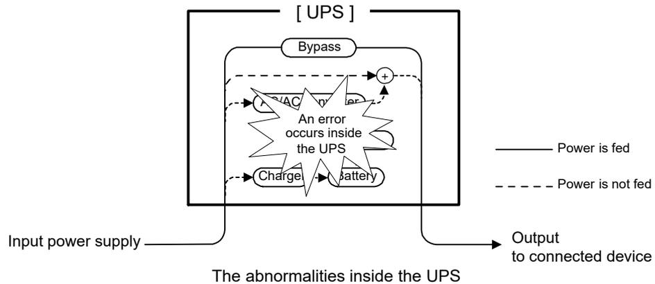
Electricity flow during automatic bypass operation
