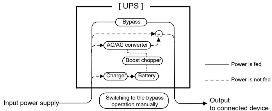
Electricity flow during automatic bypass operation
