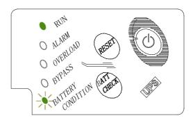
**5.** The battery check is performed for 5 seconds. Then, if the battery is normal, the BATTERY CONDITION LED (green) on the front of the UPS indicates the amount of battery charge again, and the UPS returns to the normal operation.
