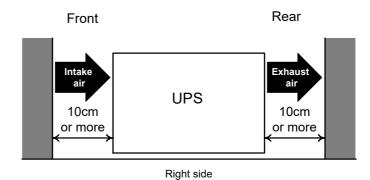
When performing maintenance on the UPS, a space of approximately 1 m is required in front of and behind the UPS.
