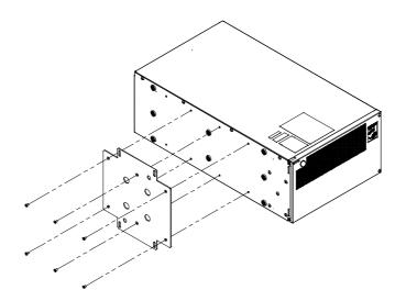
**2.** After attaching the stabilizer to the UPS, screw the stabilizer to the floor.
