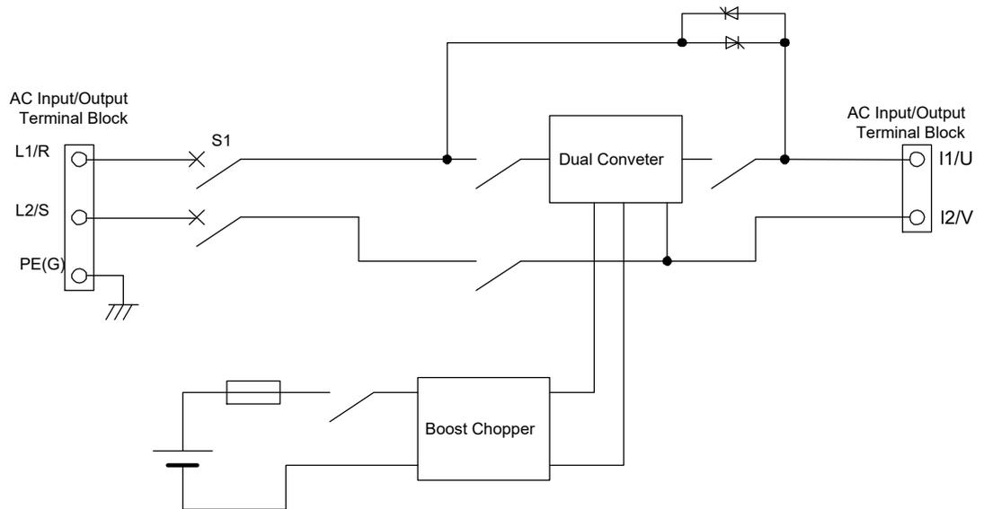
Figure 2 - Circuit diagram of Models M-UPS075AD2B-U and M-UPS100AD2B-U
