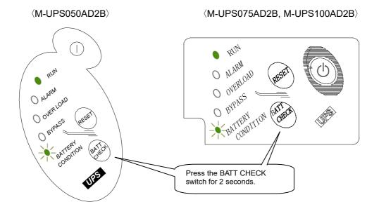
A buzzer will sound and the BATTERY CONDITION LED (orange) will flash (1.6 second cycle).
