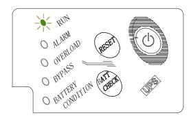
**2.** Turning on the UPS. Press the RUN/STOP switch on the front of the UPS for 1 second. The buzzer will sound when the power is on.
