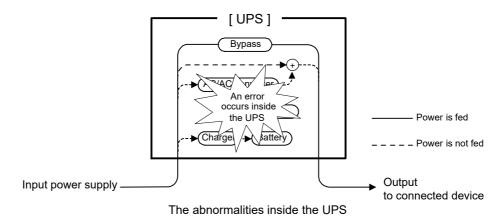
Electricity flow during automatic bypass operation
