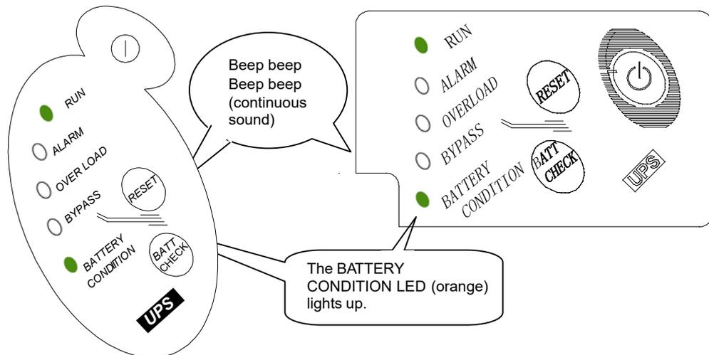
When the backup time of the battery has been lowered to 3 minutes or less (at the rated load)
