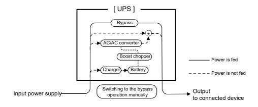
Electricity flow during automatic bypass operation
