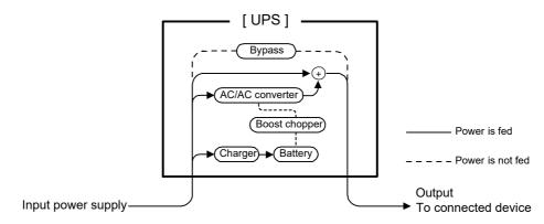
Electricity flow during normal operation
