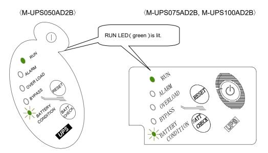
When all the LEDs on the front of the UPS are off, turn on the UPS and proceed to step 2.
