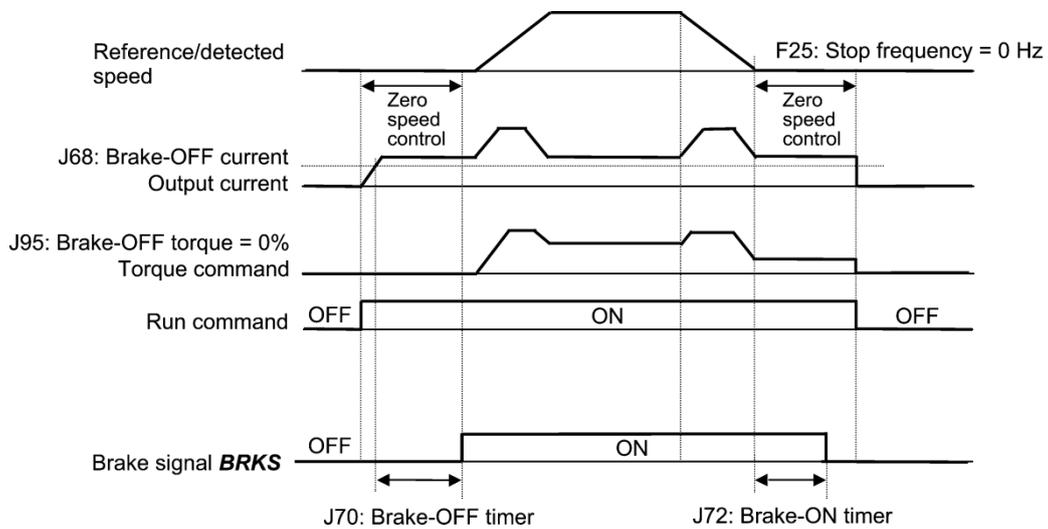
Operation time chart under vector control with speed sensor
