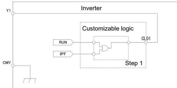
To configure this customizable logic, set the function codes as follows. (Timer selection) and (Timer setting) do not need to be modified if no change is made.
