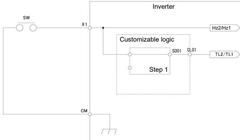
To configure this customizable logic, set the function codes as follows. (Timer selection) and (Timer setting) do not need to be modified if no change is made.
