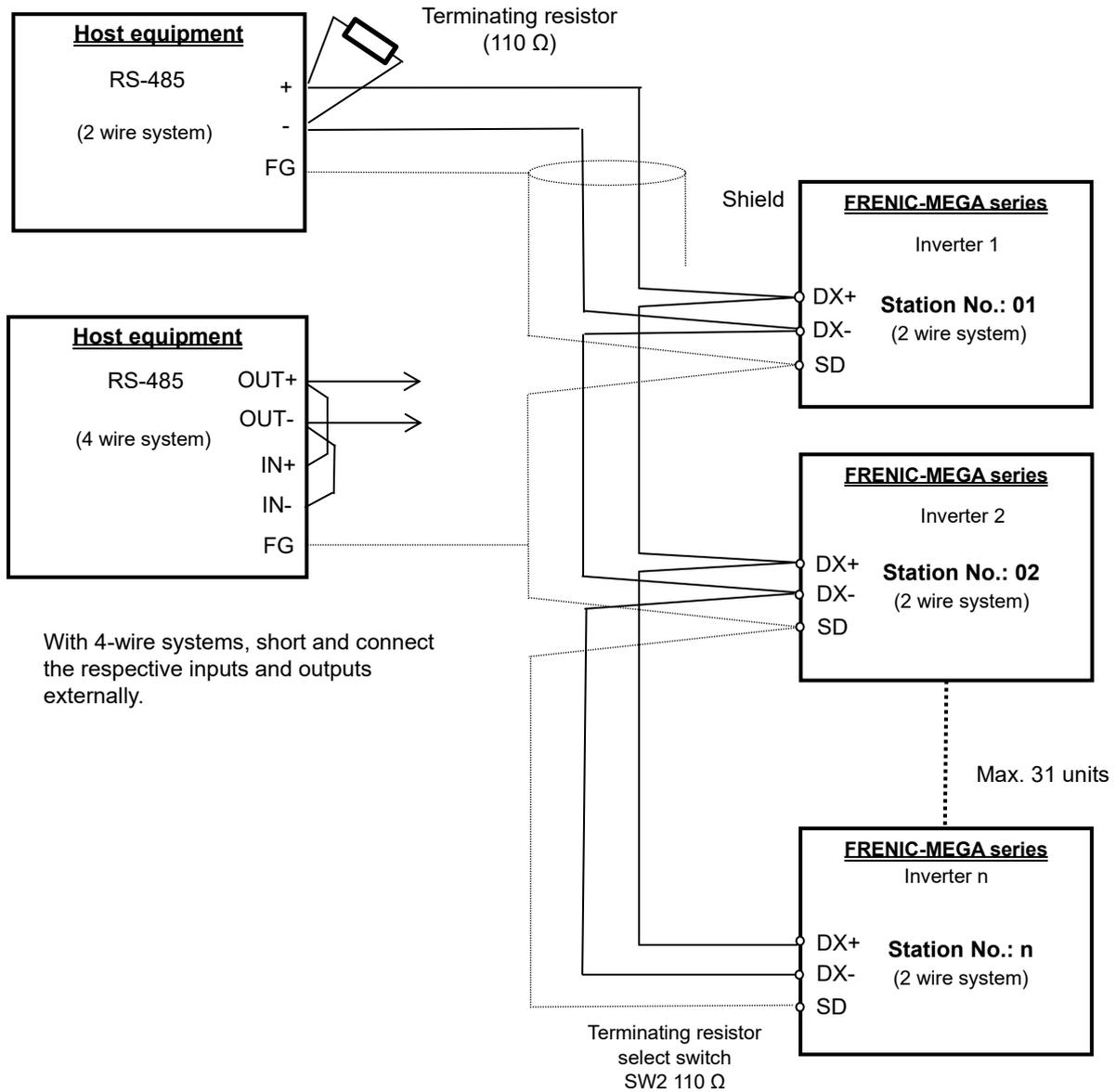
Fig. 9.1-2 Multi-drop connection diagram (terminal block connection)
