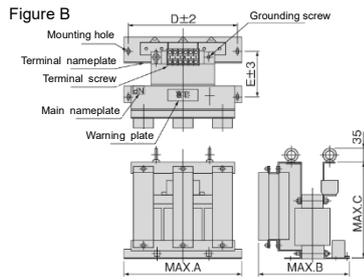
■ Filter dimensions (30 kW or higher): reactors
