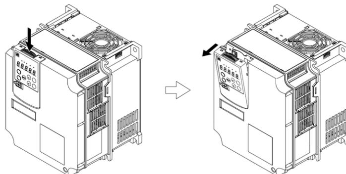
Fig. 2.3-2 Keypad removal
