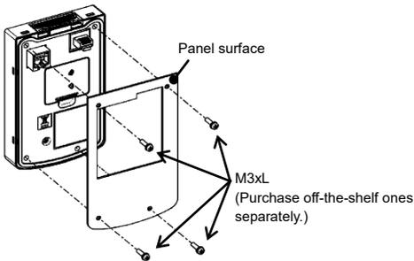
Figure 2.3(a) Keypad installation
