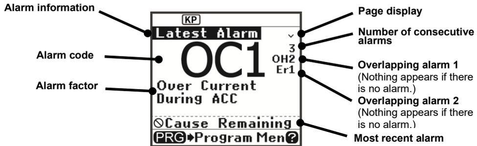
Fig. 3.1-4 Screen samples in running and alarm modes
