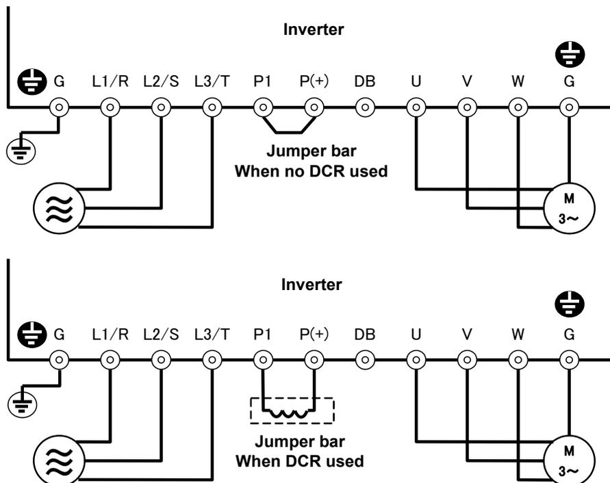
Fig. 4.2-1 Connection of main circuit terminals (three-phase power supply)
