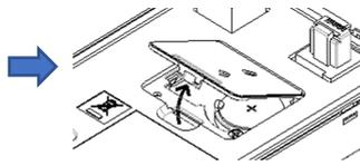
With the slit pushed up, lift up the back cover in the arrow direction (approx. 45°)
