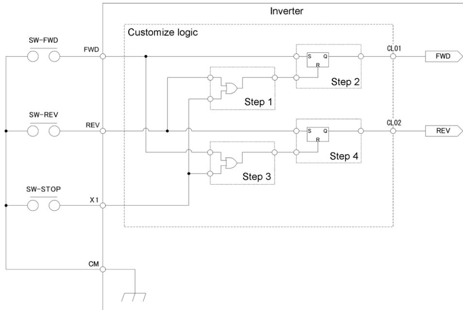
To configure this customizable logic, set the function codes as follows. (Timer selection) and (Timer setting) do not need to be modified if no change is made.
