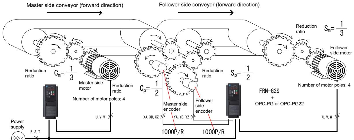
Master-follower operation system configuration example (with Z-phase compensation)
