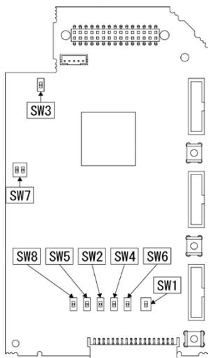
Fig. 2.2-25 Switch positions
