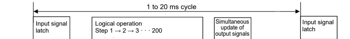
The step execution order for multi-tasks is shown in the following diagram.
