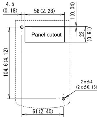
Figure 2.2(b) Panel cutout size drawing (when reusing panel cutout for previous product)
