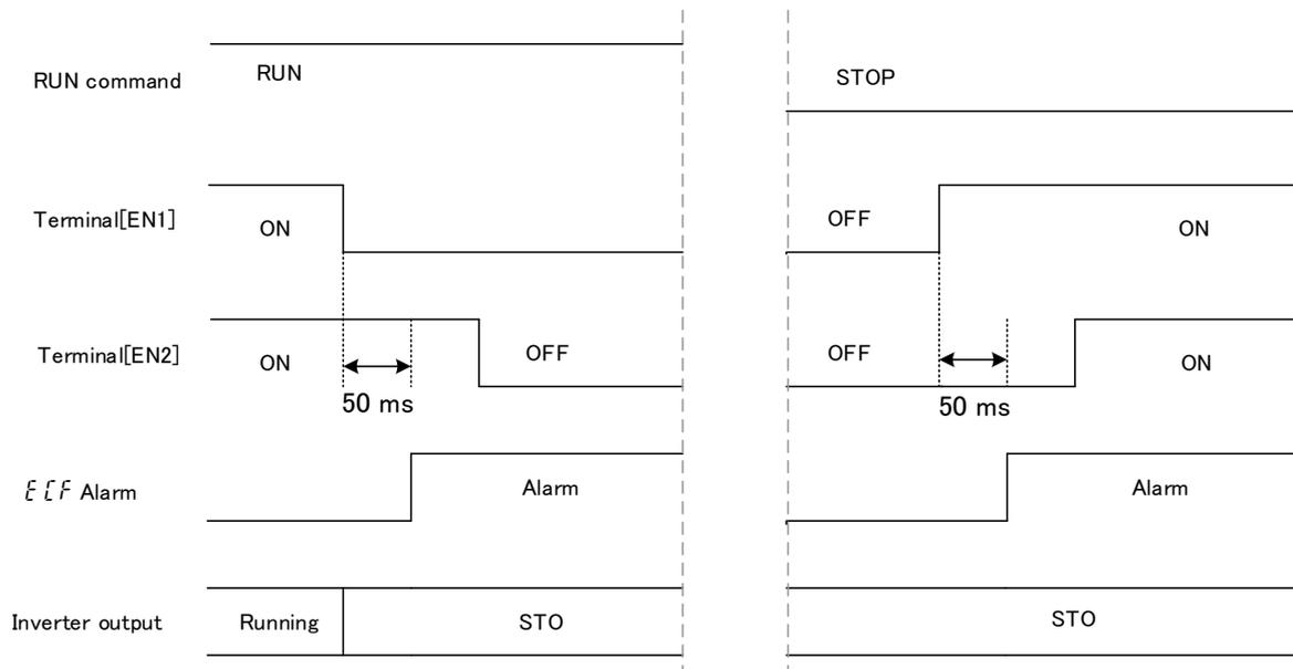
Fig. G. 4-4  $\overline{E} \overline{L} \overline{F}$  alarm (logical mismatch) and inverter-output status
