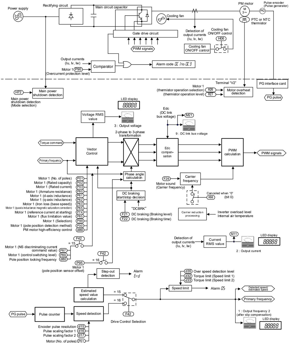
Fig. 8.9-10 Vector control (PMSM drive 2) section block diagram
