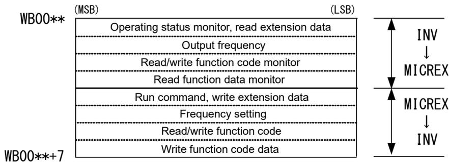
Note) \*\* is the T-link bus station No. set with "RSW1" and "RSW2".
