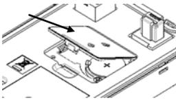
Align the 2 clips on the back cover with the panel, and insert in the arrow direction.
