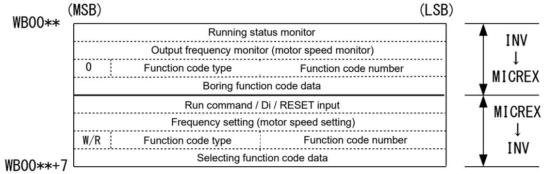
Note) \*\* is the T-link bus station No. set with "RSW1" and "RSW2".
