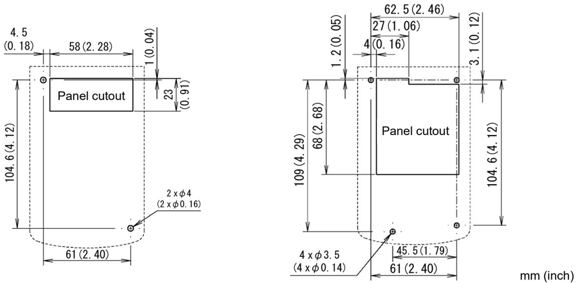
When using previous compatible panel cutting
