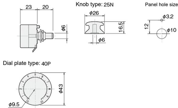
(Note) The nameplate and dial must be ordered separately (parts available from Fuji Electric Technica Co., Ltd.)
