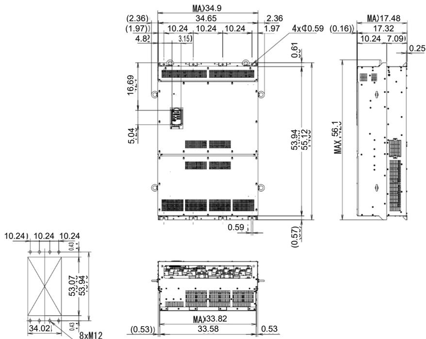
Panel cutout size drawing for external cooling installation
