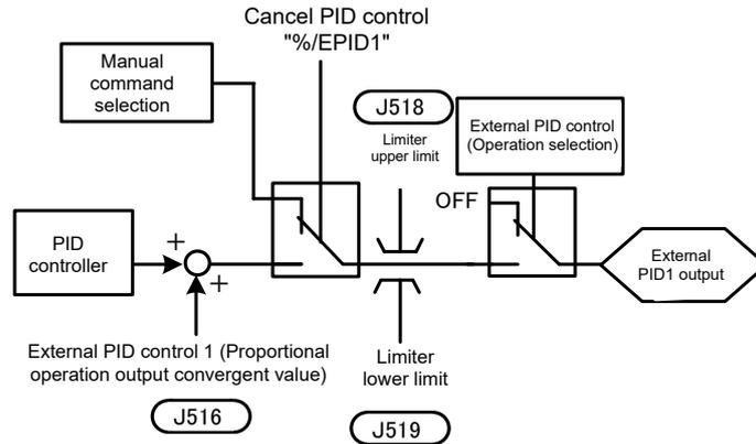
Furthermore, the following proportional operation is possible by disabling I (Integral time) and D (Differential time), and setting for P (Gain) and this value only.
