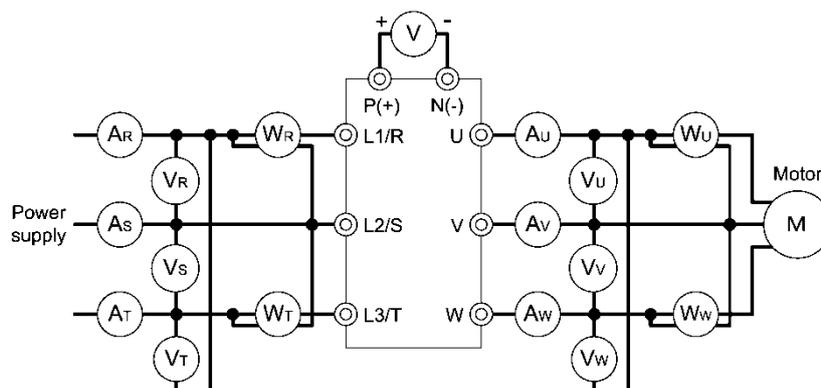
Fig. 7.5-1 Connection of meters
