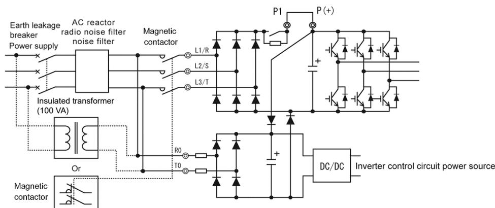
Fig. 2.2-10 Earth leakage circuit breaker connection
