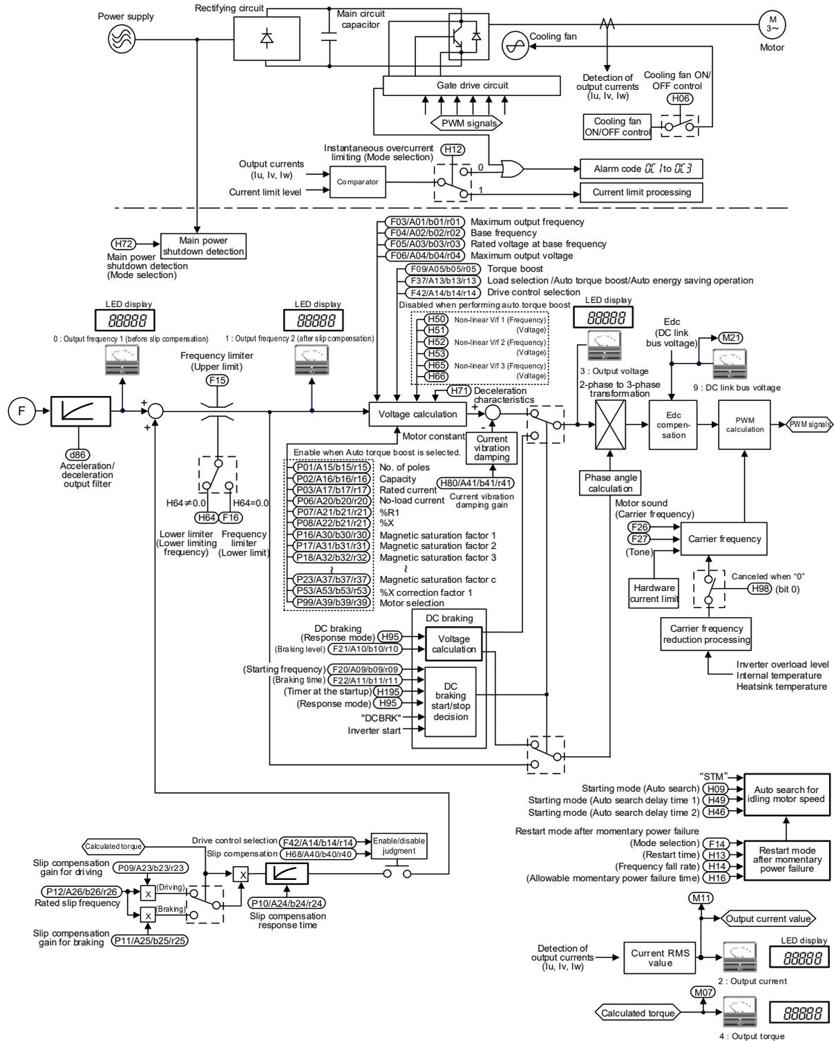
Fig. 8.9-2 V/f control (without speed feedback) section block diagram
