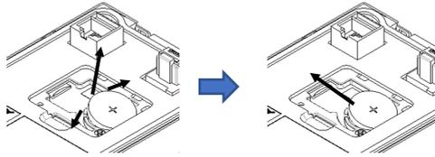
Hold open the 2 securing clips on the left side of the battery, and lift up the battery. Take care not to let the battery pop out.
