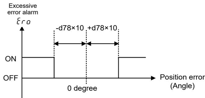
Excessive error alarm  $E_{rD}$
