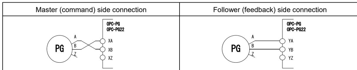
(Note 1) With speed synchronization, there is no need to connect to terminal [XZ] and [YZ].
