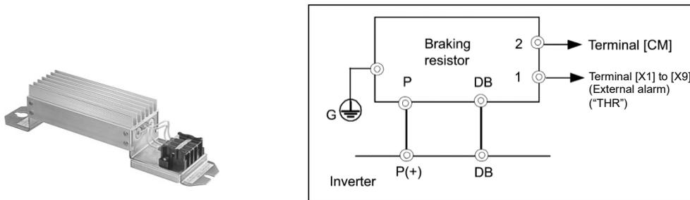
Fig. 11.6-2 Braking resistor (standard type) and connection example
