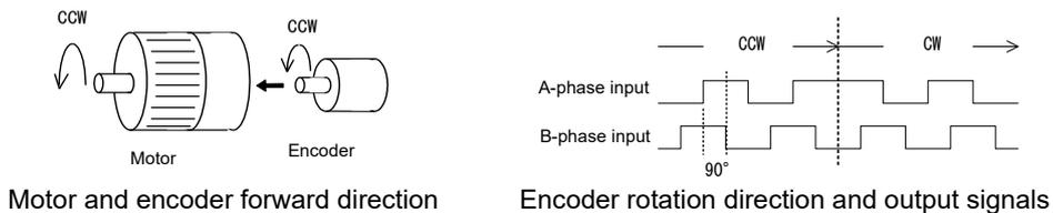
Motor and encoder forward direction
