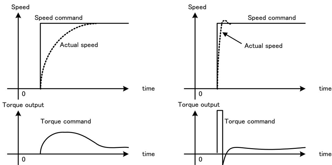
The above mentioned effect can be obtained by setting the P gain of ASR higher. However the response of the system becomes faster in this setting and there is the possibility that it affects negatively due to generation of vibration.
