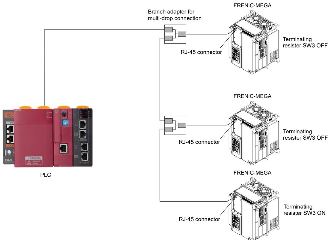
Fig. 9.1-1 Multi-drop connection diagram (RJ-45 connector connection)
