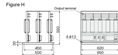
Table 11.11-2 Filter for output circuit (external dimensions)
