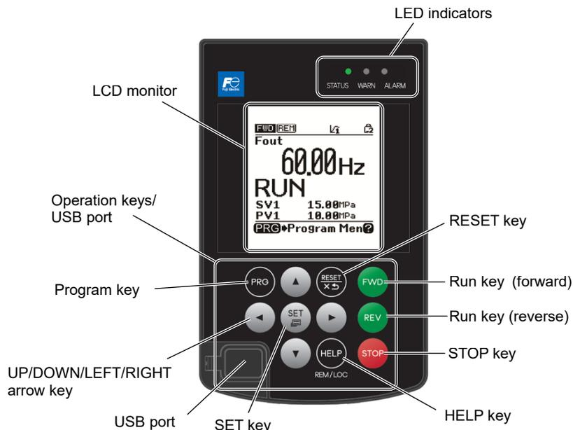
Fig. 3.1-3 Names and functions of keypad components
