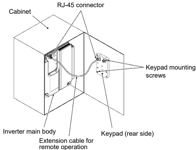
Fig. 2.3-1 If installing the keypad on the panel
