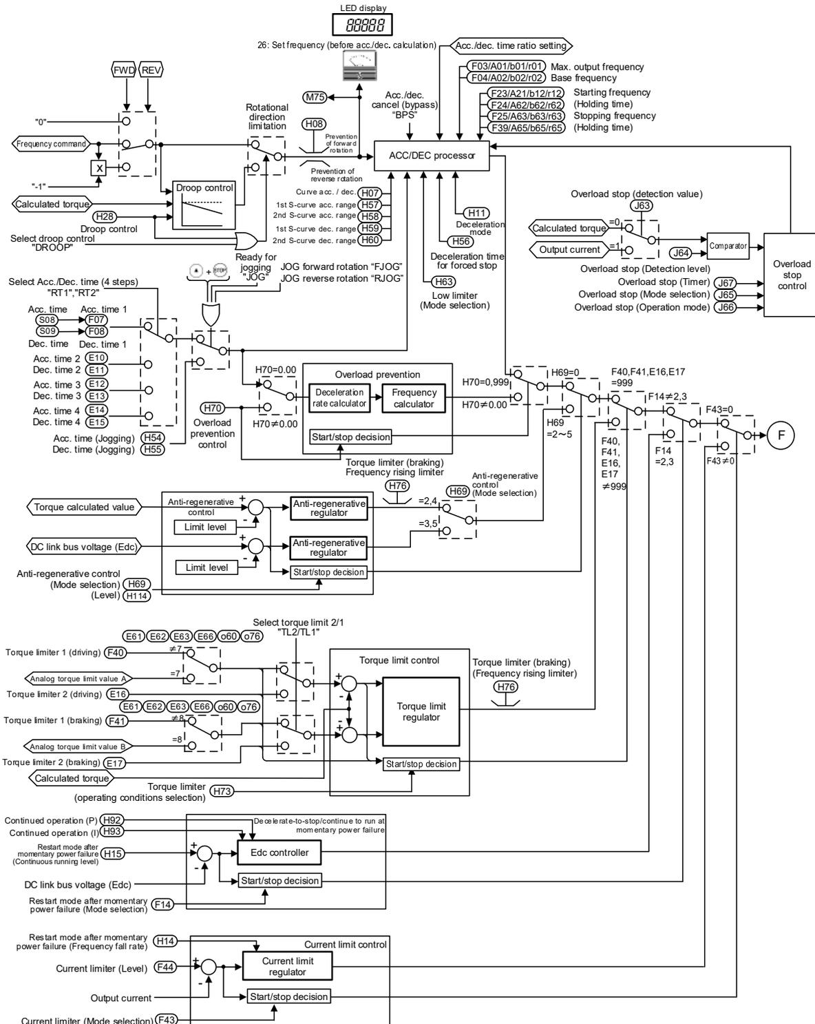
Fig. 8.9-1 V/f control (common) section block diagram
