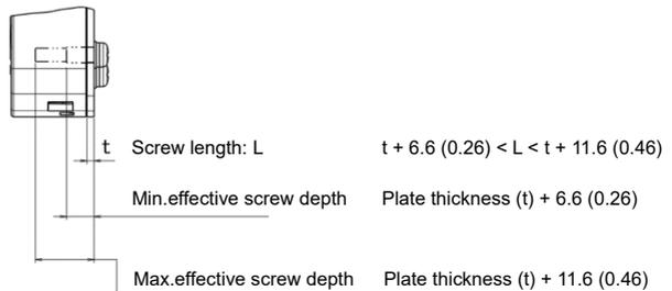
Note: There is a risk of keypad damage if using a screw with maximum effective screw depth or greater.
