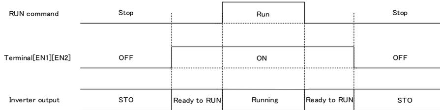
Fig. G.4-2 Inverter output status when terminal [EN1], [EN2] is turned OFF while the inverter is stopped
