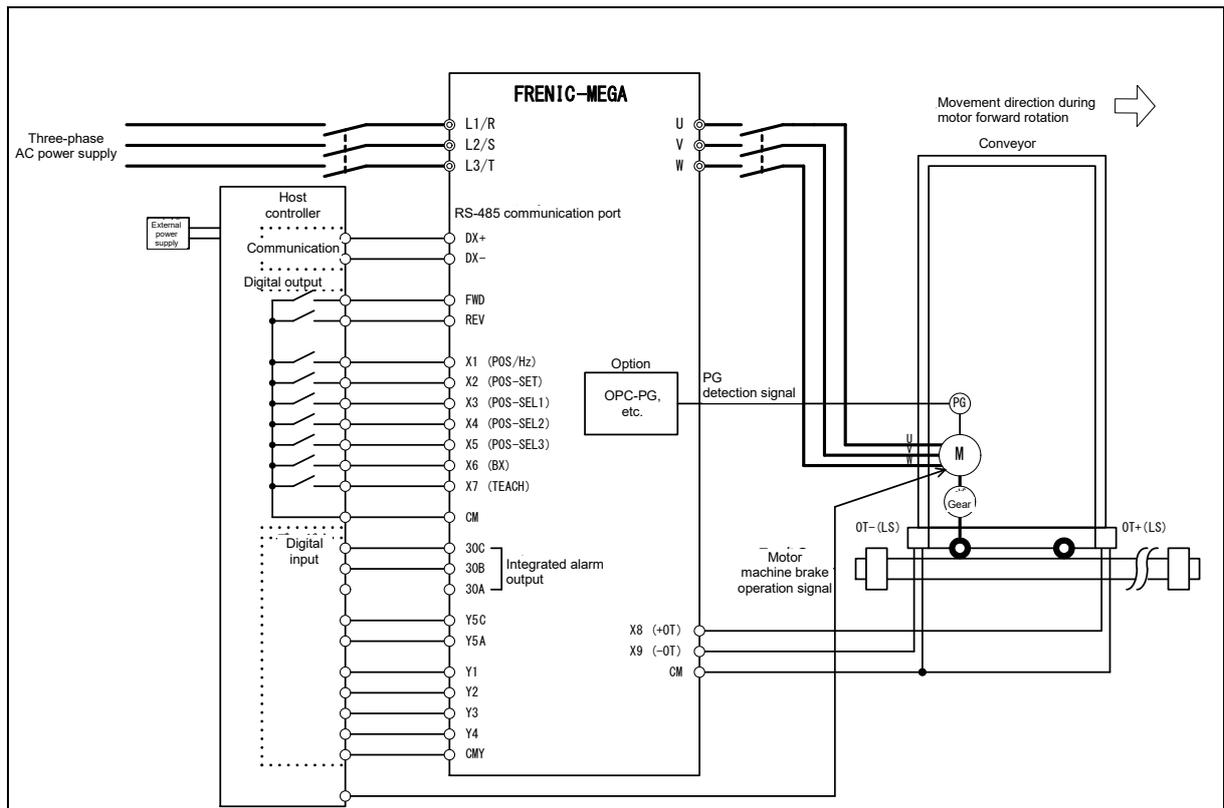
**Note** Do not set direction limit [H08] to 1 or 2 when performing position control. Position control will not function normally.
