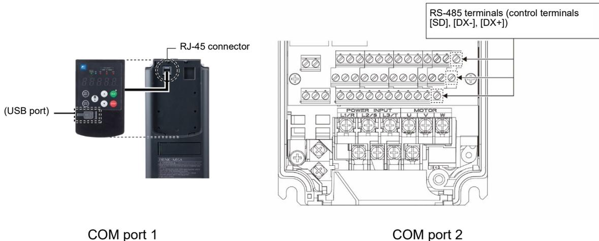
Using the RS-485 COM ports shown above enables the extended functions listed below.
