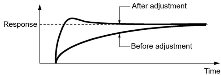
3) Suppressing oscillation for cycles longer than the integral time set in the function code J511, J611, and J661 data
