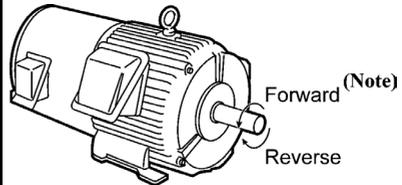
**(Note)** The rotation direction of IEC-compliant motors is opposite to that of the motor shown here.
