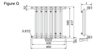
The reactor, and resistors and capacitors are separately installed on OFL-30-4A or higher models. (If ordering a filter type, reactors, resistors, and capacitors are shipped as a set.)
