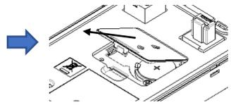
Remove the back cover in the arrow direction.
