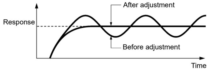
4) Suppressing oscillation for cycles roughly the same as the differential time set in the function code J512, J612, and J662 data
