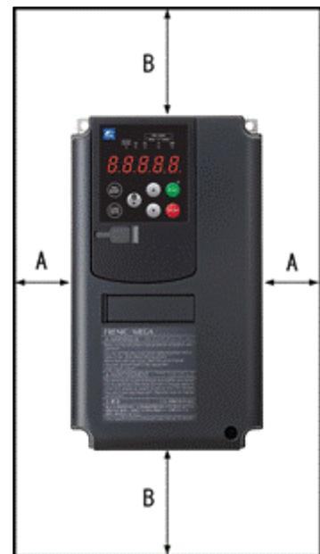
Fig. 2.1-1 Installation direction
