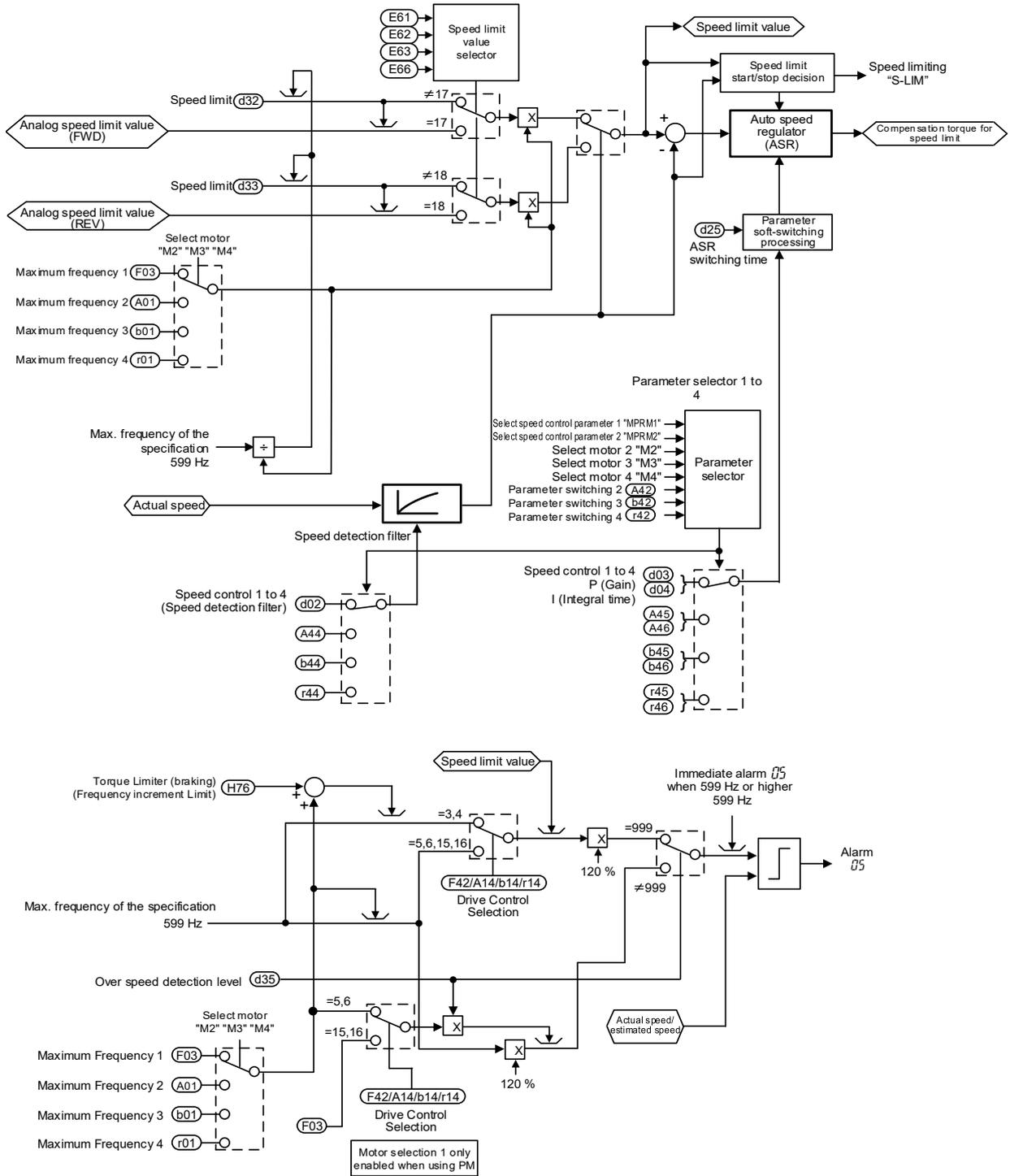
Fig. 8.9-7 Vector control (speed control / over speed protection processing) section block diagram
