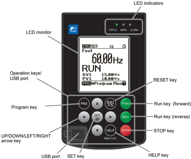
Figure 3.1 Names and Functions of Keypad Components
