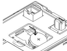
Push the battery down. (it will fit into securing clips, making snapping sound)
