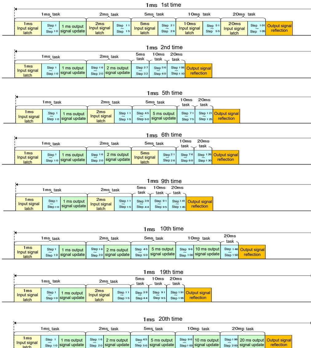
Note that if you do not consider the process order of customizable logic when configuring a function block, the expected output may not be obtained, the operation can be slower or a hazard signal can occur, because the output signal of a step is not available until the next cycle.
