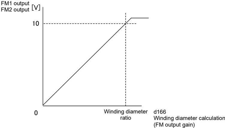
If outputting the winding diameter ratio to terminal [FM1] and [FM1], set 25 for function code F31 and F61, respectively. The gain can be adjusted even with function code F30 and F60 for terminal [FM1] and [FM2] side.
