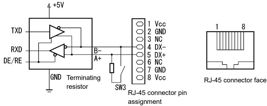
**Note** The power supply for the keypad (pins 1, 2, 7, and 8) is connected to the RJ-45 connector for RS-485 communication (standard). When connecting other devices to the RJ-45 connector, take care not to use those pins. Use pins **4 and 5 only**.
