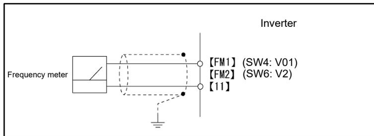
Fig. 11.17-1 Frequency meter external dimensions and connection example
