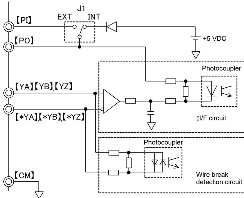
Fig. 11.19-14 Circuit configuration
