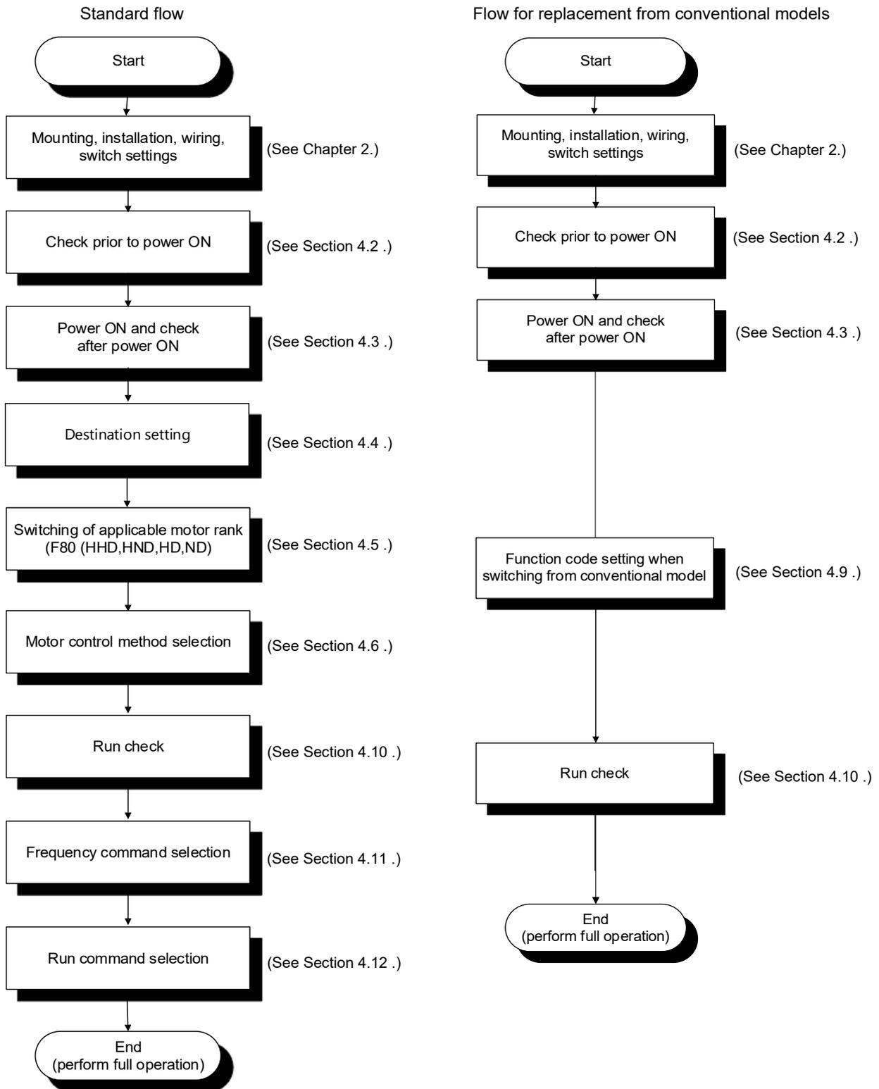
Fig. 4.1-1 Test run procedure
