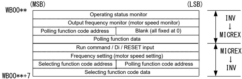
Note) \*\* is the T-link bus station No. set with "RSW1" and "RSW2".
