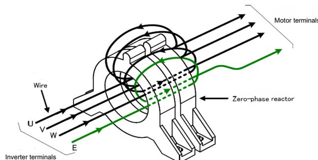
Fig. 11.12-2 Connection example for 2 reactors x 2 turns = 4 turns
