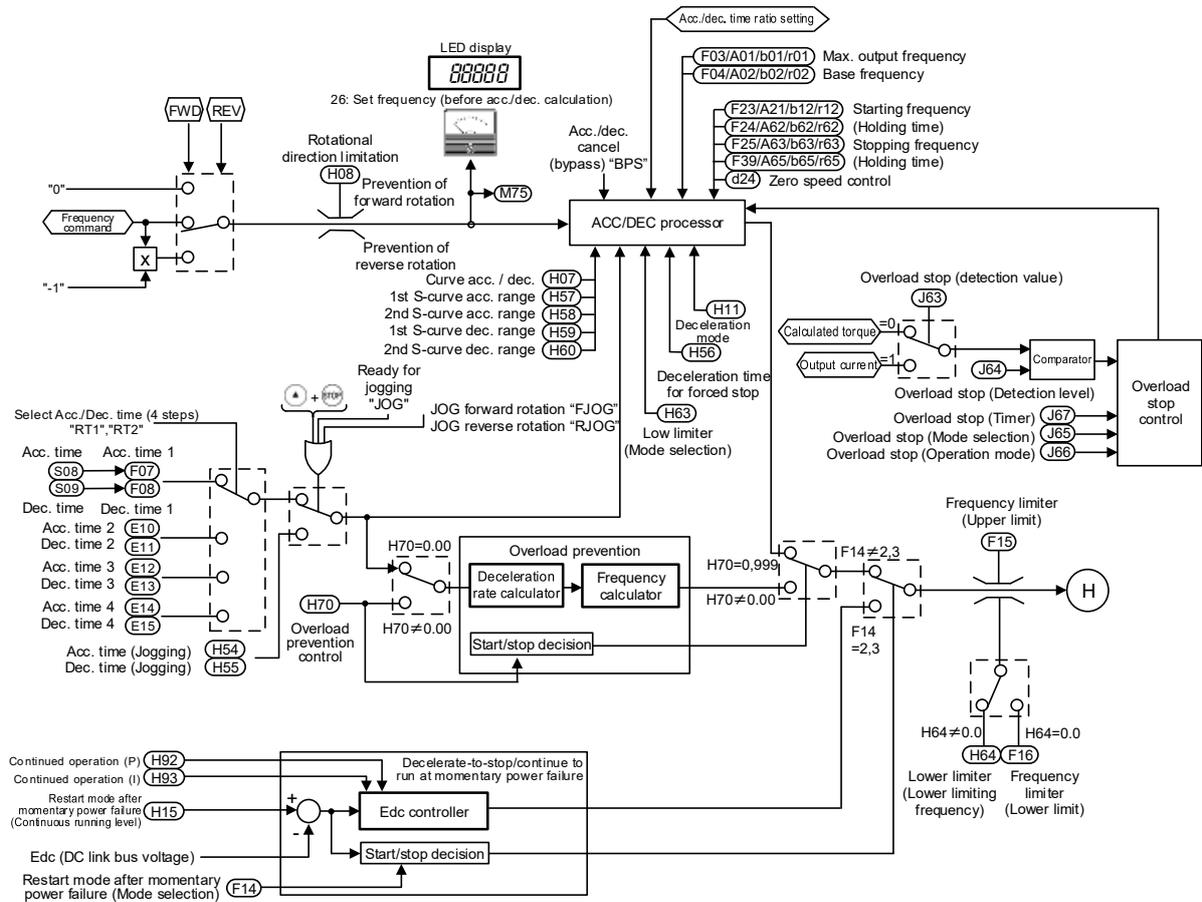
Fig. 8.9-4 Vector control (common) section block diagram
