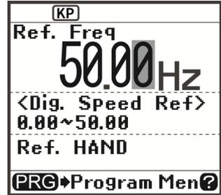
Figure 3.4 Setting up Frequency Command (display sample)
