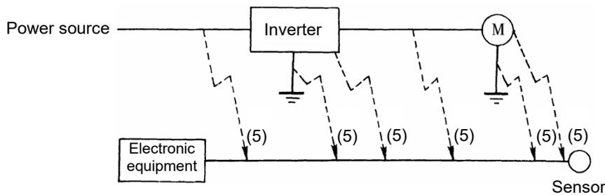
Fig. A.2-6 Radiated noise
