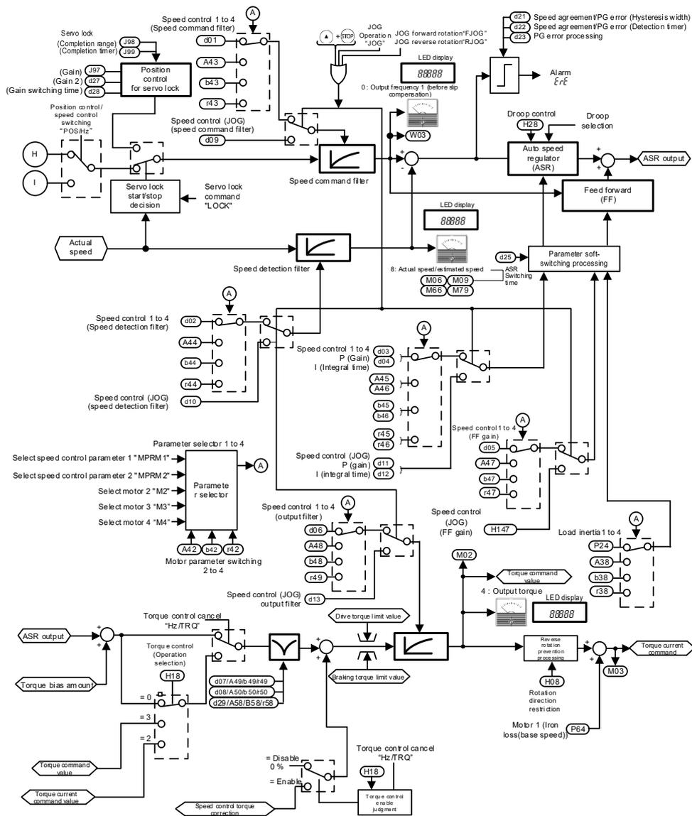
Fig. 8.9-9 Vector control (PMSM drive 1) section block diagram
