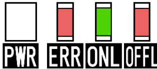
Figure 2.6 LED Status Indicators
