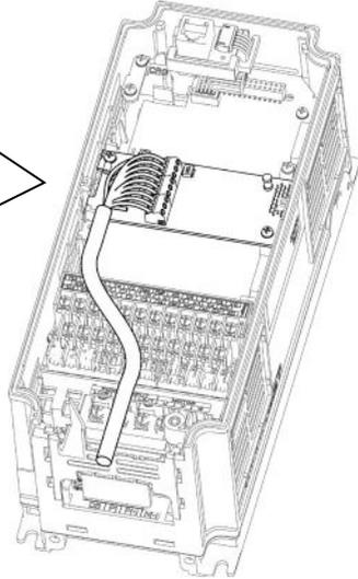
\* Pass the wires from the interface card between the control circuit terminal block and the front cover.
