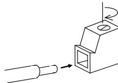
Figure 1.7 Connecting to a Terminal on Interface Card
