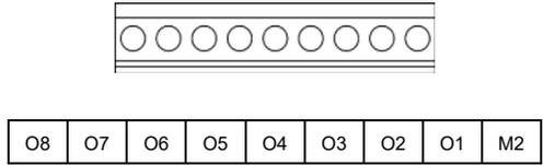
Figure 3.1 Terminal Allocation and Symbol Diagram
