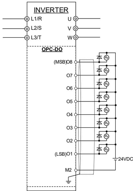
Figure 3.2 Connection Diagram
