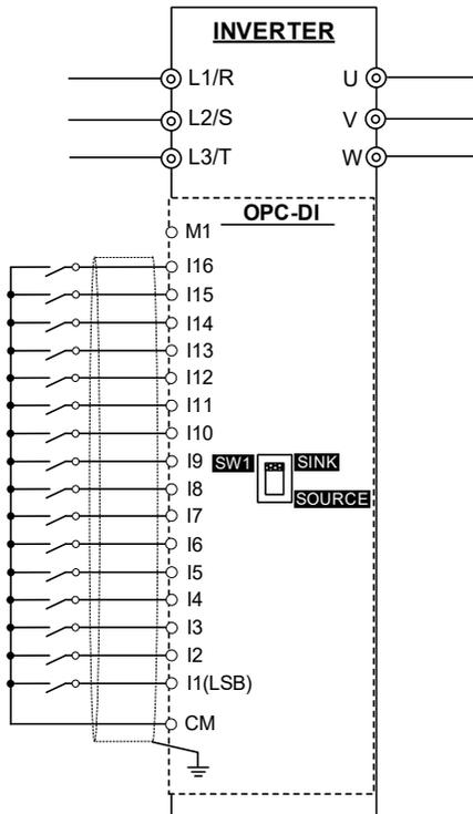
Figure 2.2 Connection Diagram
