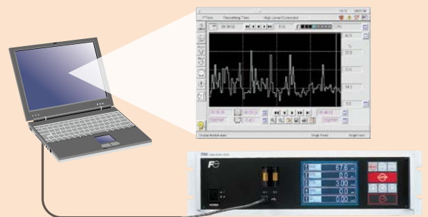
RS-485 (Modbus) communication
